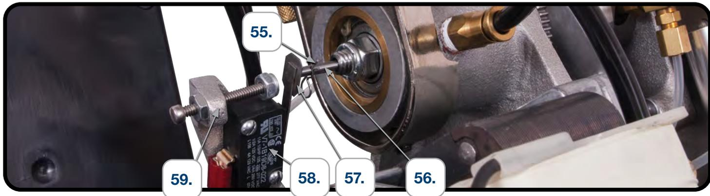
55. Trigger Rod Retaining Clip [64090]
