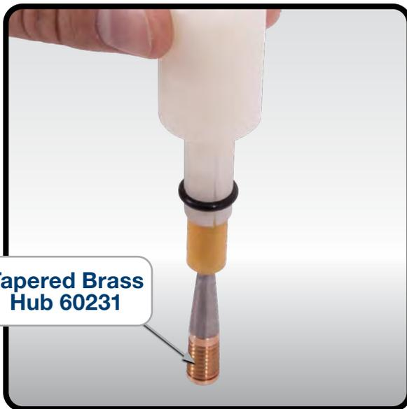
3. Force sleeve down onto tool shaft
